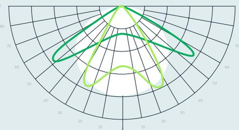
The 120 degree optic is the ideal choice for vertical and indoor applications where the lights need to be mounted at a height between 6" and 36", providing an equal distribution of light over the canopy.
