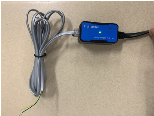
Inputting RJ9 Pin Connector into the Type F Lighting Adapter.
