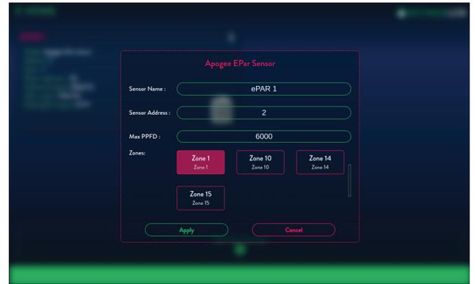
**Zones:** Indicates the active zones on the Echo Display. Select the zone this sensor should control.
